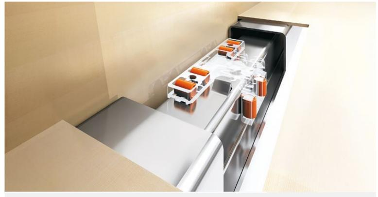
The Blum technology behind the feather-light glide: roller carriage with low-friction nylon rollers and a smooth transition between profiles to reduce noise.
